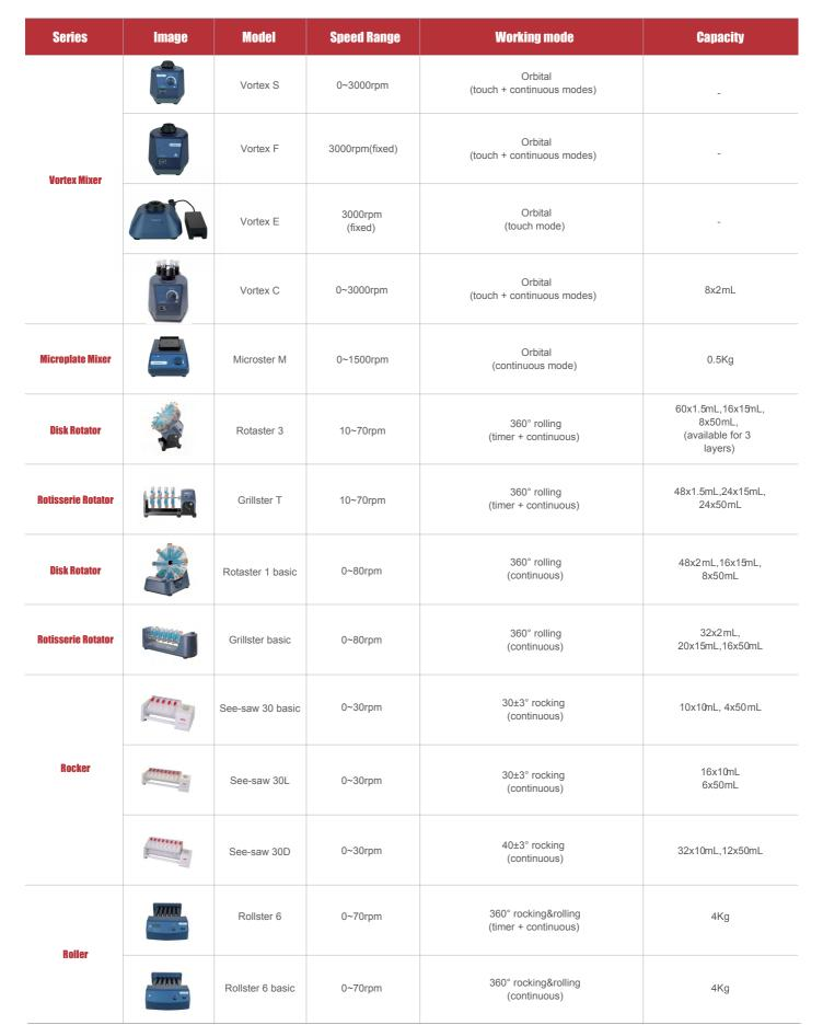
Lab1st mixers range can be divided into different series as per mixing speed, working mode, load capacity etc:
